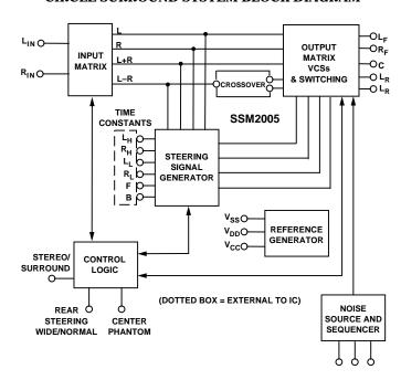
tificial ambiance or reverberation, nor does it require any delay generators. The fully differentiated rear channels provide rear stereo separation for enhanced spacial perception while maintaining full bass response, especially important in automotive applications.
