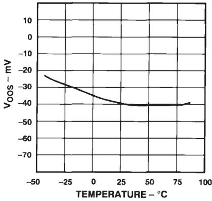
Figure 15.  $V_{oos}$  vs. Temperature
