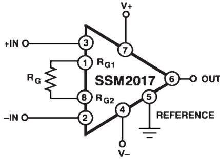
$$G = \frac{V_{OUT}}{(+In) - (-In)} = \left( \frac{10\text{ k}\Omega}{R_G} \right) + 1$$
