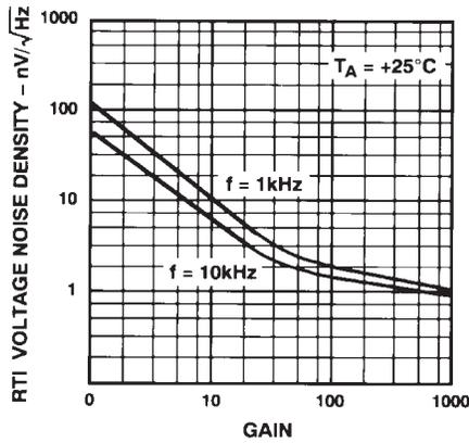
Figure 4. RTI Voltage Noise Density vs. Gain
