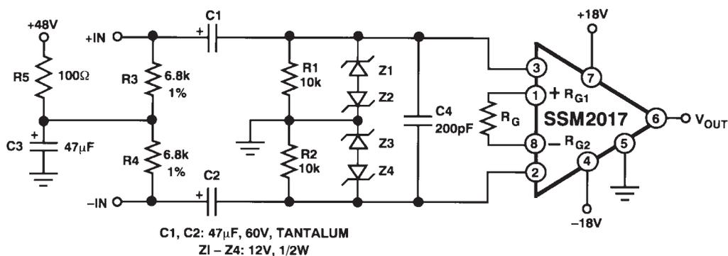
Figure 23. SSM2017 in Phantom Powered Microphone Circuit
