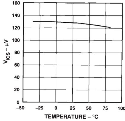
Figure 13.  $V_{los}$  vs. Temperature
