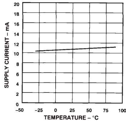
Figure 19.  $I_{sy}$  vs. Temperature
