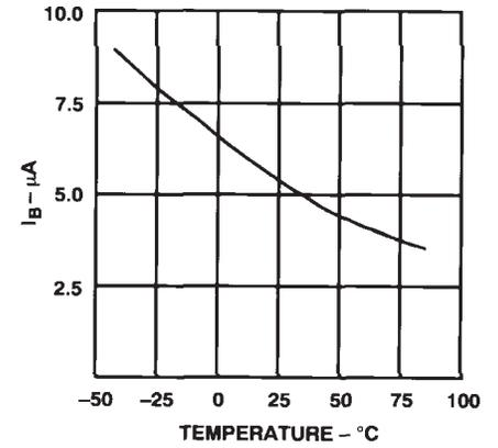
Figure 17.  $I_B$  vs. Temperature
