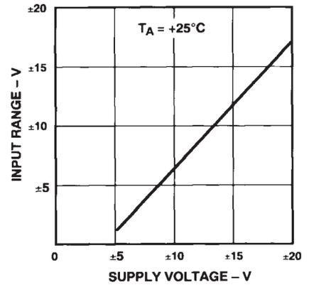
Figure 8. Input Voltage Range vs. Supply Voltage
