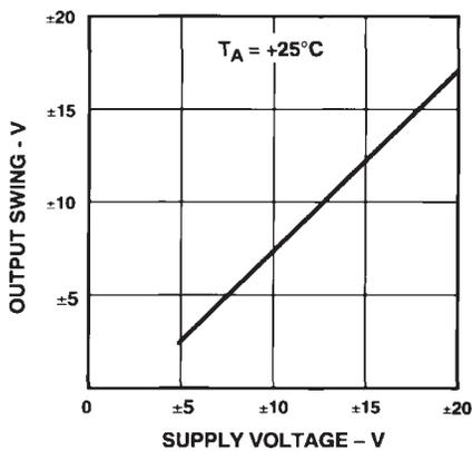
Figure 9. Output Voltage Range vs. Supply Voltage
