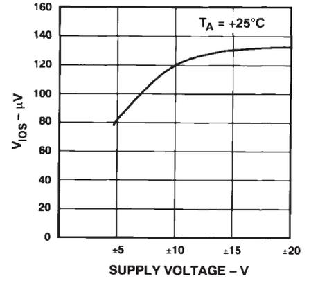
Figure 14.  $V_{los}$  vs. Supply Voltage
