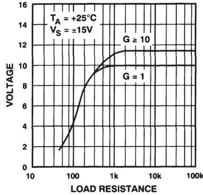
Figure 7. Maximum Output Voltage vs. Load Resistance
