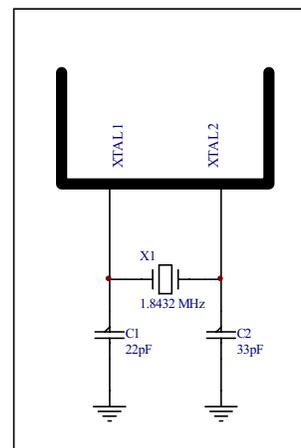
the XTAL1 pin to clock the internal baud rate generator for standard or custom rates. (see Baud Rate Generator Programming).
