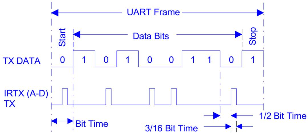
Infrared transmit timing
