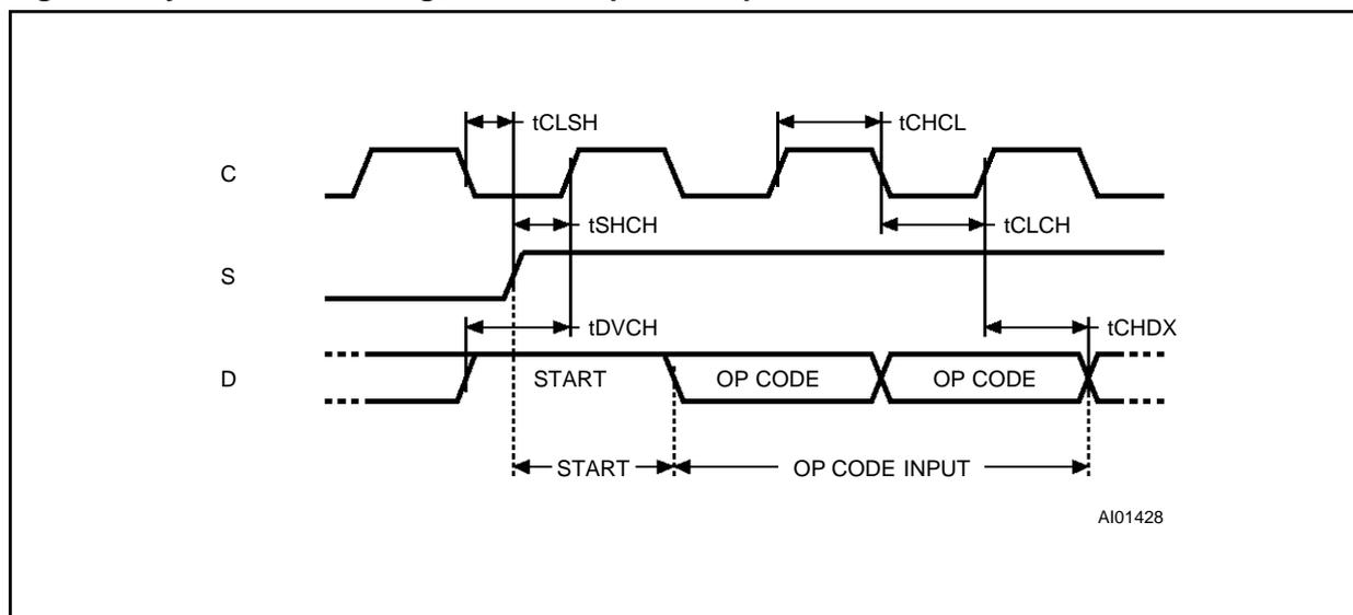
Figure 5. Synchronous Timing, Read or Write
