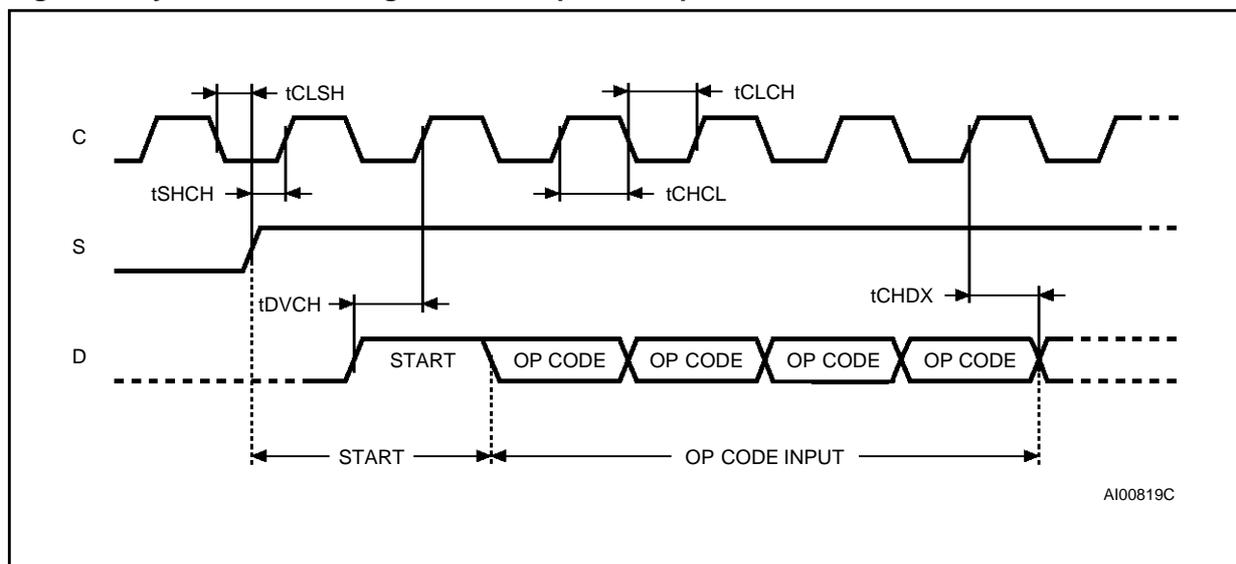
Figure 5. Synchronous Timing, Read or Write
