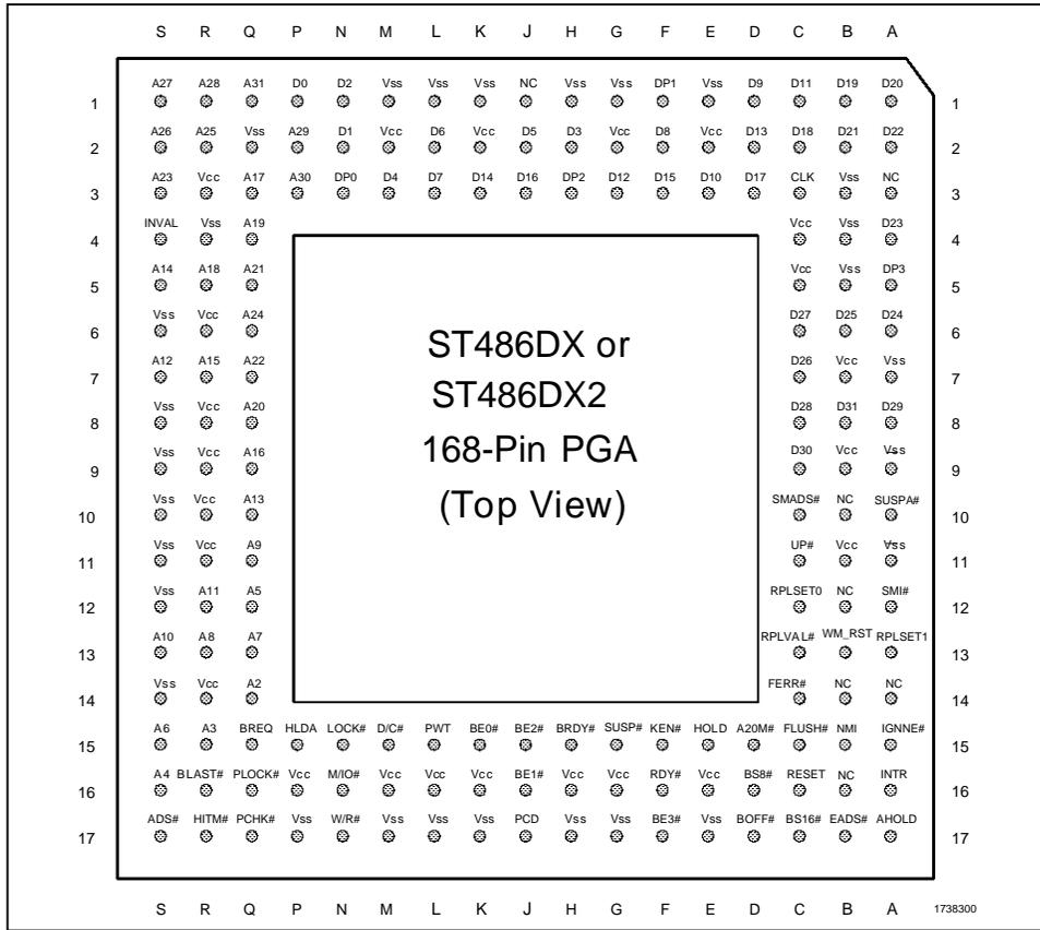
Figure 3 - 1. 168-Pin PGA Package Pin Assignments
