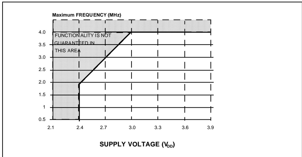
The shaded area is outside the recommended operating range; device functionality is not guaranteed under these conditions.
