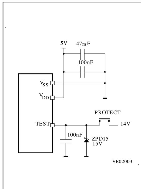
Note: ZPD15 is used for overvoltage protection
