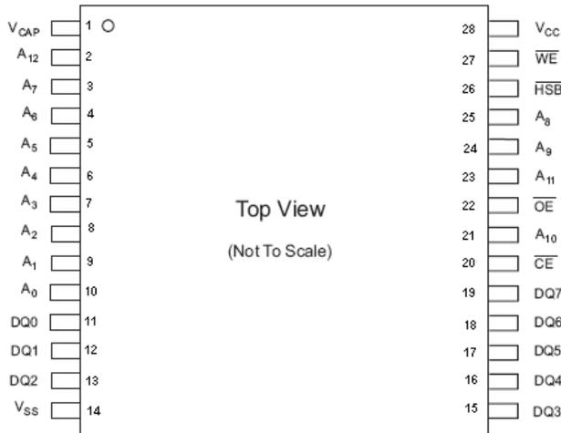
Figure 2. Pin Diagram - 28-Pin LLC
