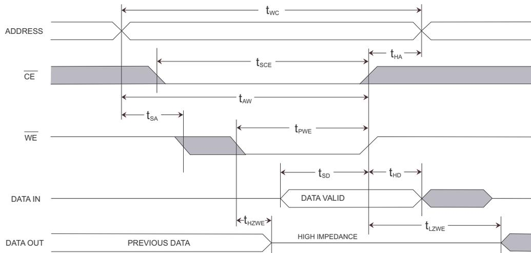
**Figure 11. SRAM Write Cycle 2:  $\overline{CE}$  Controlled** [13, 14]
