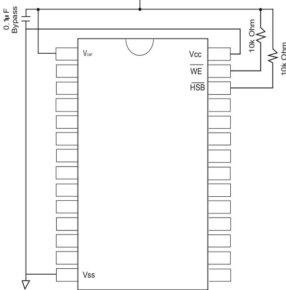
If the power supply drops faster than 20  $\mu\text{s}/\text{volt}$  before  $V_{CC}$  reaches  $V_{SWITCH}$ , then a 2.2  $\Omega$  resistor must be connected between  $V_{CC}$  and the system supply to avoid momentary excess of current between  $V_{CC}$  and  $V_{CAP}$ .
