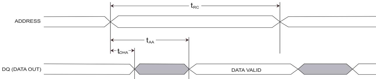
Figure 9. SRAM Read Cycle 2:  $\overline{CE}$  and  $\overline{OE}$  Controlled <sup>[7]</sup>
