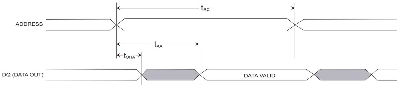
Figure 6. SRAM Read Cycle 2:  $\overline{CE}$  and  $\overline{OE}$  Controlled [5]
