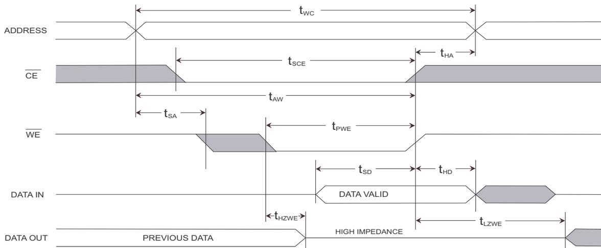
Figure 8. SRAM Write Cycle 2:  $\overline{CE}$  Controlled [8]
