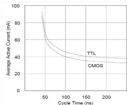
Figure 3. Current Versus Cycle Time (READ)
