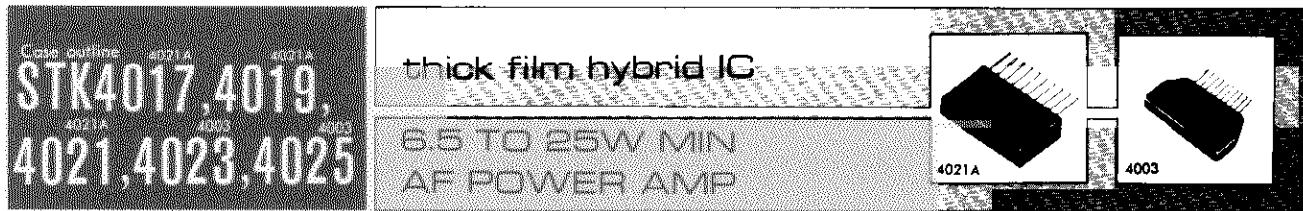
Fabricated on the IMST substrate of our own originality and designed for use in intermediate-power, single-channel, single-supply voltage amplifiers. Their packages are made much more compact than those of the Type Nos. heretofore in use, thereby meeting the requirements for making the set smaller and slimmer. They are especially suited for use in electronic organs or electric pianos.
