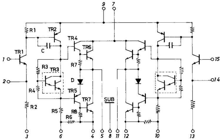
Sample Application Circuit: 25W min 2-Channel AF Power Amplifier
