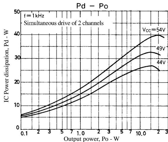
Figure 1. STK4432 Pd - Po (R<sub>L</sub> = 8Ω)
