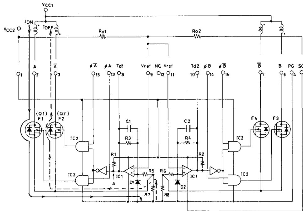
Fig. 1 STK6712AMK3 Internal Equivalent Circuit
