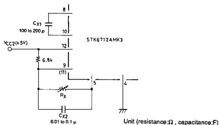
Fig. 10 Motor Hold Noise Countermeasure
