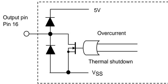
(The buffer has an open drain configuration.)
