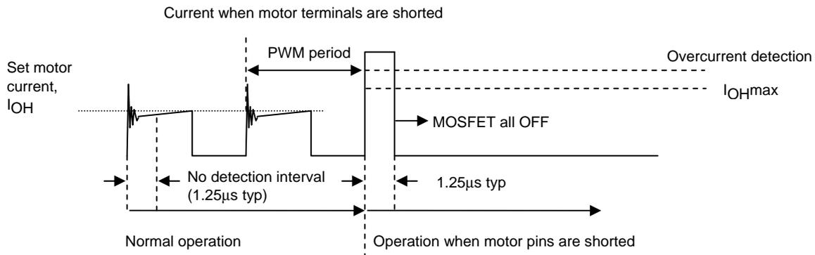
Overcurrent detection begins after an interval of no detection (a dead time of 1.25 $\mu$ s typ) during the initial ringing part during PWM operations. The no detection interval is a period of time where overcurrent is not detected even if the current exceeds  $I_{OH}$ .
