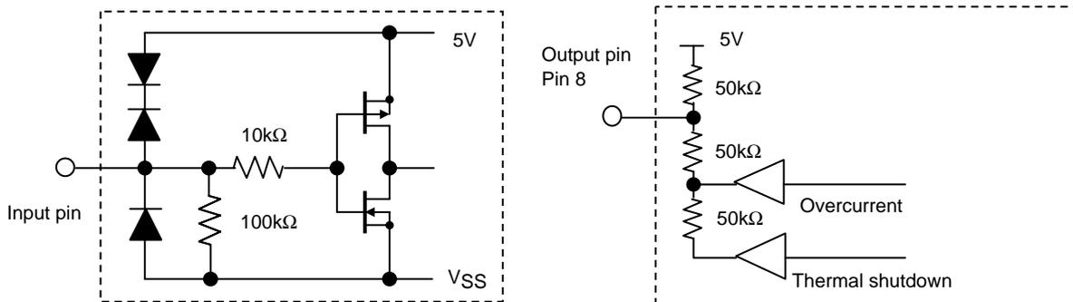
The input pins of this driver all use Schmitt input. Typical specifications at  $T_c=25^\circ\text{C}$  are given below. Hysteresis voltage is 0.3V ( $V_{IHa}-V_{ILa}$ ).
