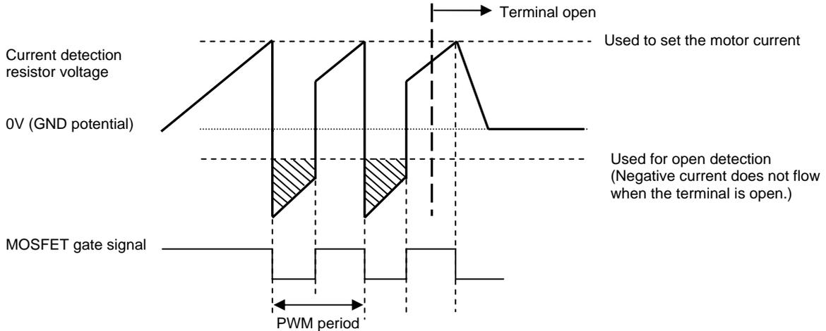
When the current level drops, the difference with the GND potential decreases, making detection difficult. The motor current that can be detected by motor terminal open detection is 1.1A or more with the STK672-432B-E and 1.4A or more with the STK672-442B-E/440B-E.
