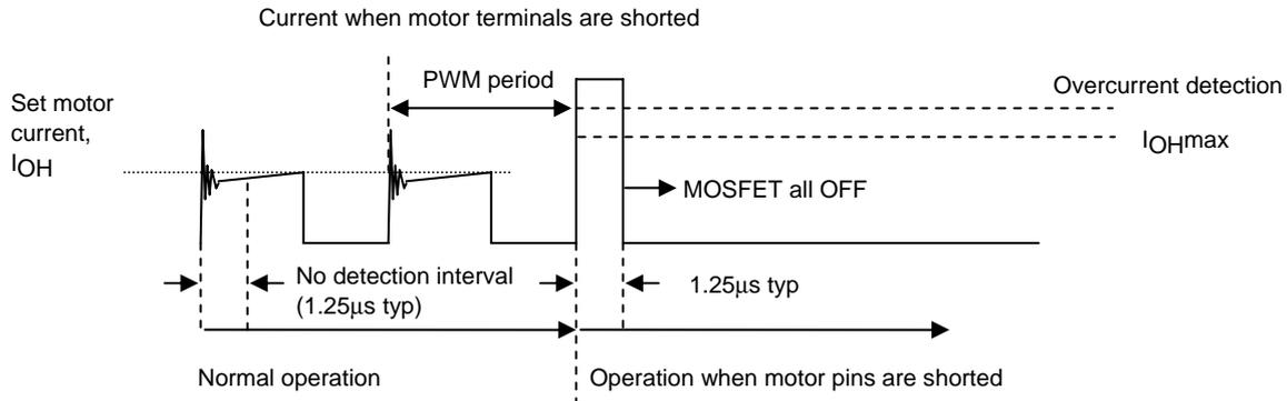
Overcurrent detection begins after an interval of no detection (a dead time of 1.25μs typ) during the initial ringing part during PWM operations. The no detection interval is a period of time where overcurrent is not detected even if the current exceeds I<sub>OH</sub>.
