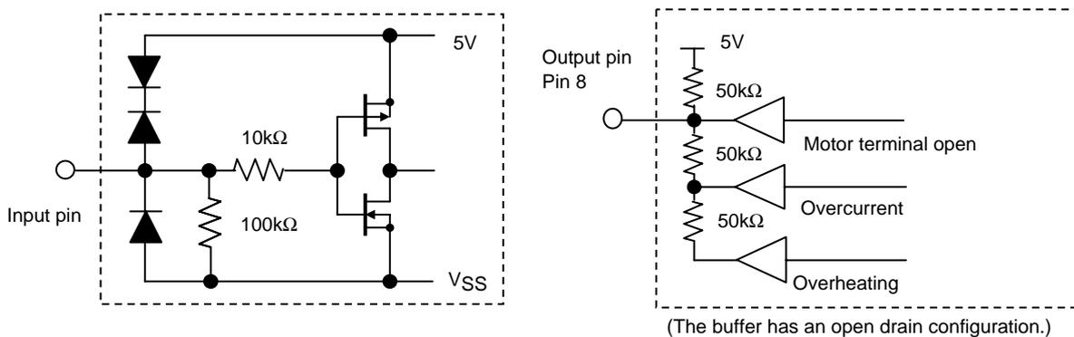
The input pins of this driver all use Schmitt input. Typical specifications at  $T_c=25^\circ C$  are given below. Hysteresis voltage is 0.3V ( $V_{IHa}-V_{ILa}$ ).
