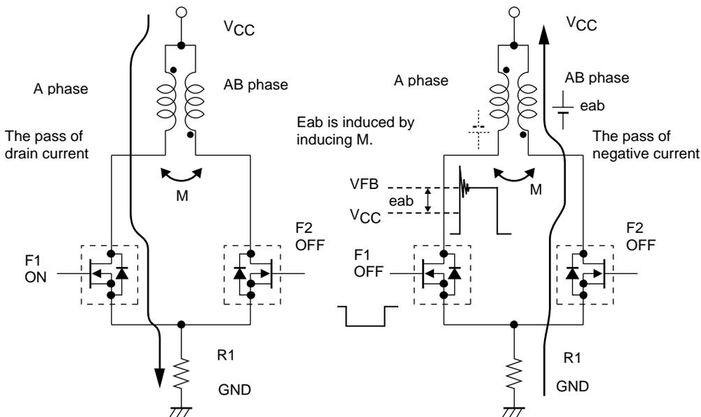
The oscillating voltage in excess of  $V_{FB}$  is caused by LCRM (inductance, capacitor, resistor, mutual inductance) oscillation that includes micro capacitors C, not present in the circuit. Since M is affected by the motor characteristics, there is some difference in oscillating voltage according to the motor specifications. In addition, constant voltage drive without constant current drive enables motor rotation at  $V_{CC} \geq 0V$ .
