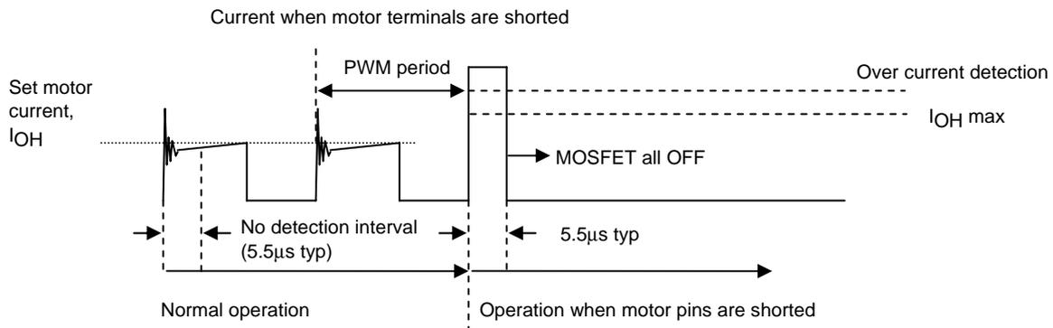
Over current detection begins after an interval of no detection (a dead time of 5.5μs typ) during the initial ringing part during PWM operations. The no detection interval is a period of time where over current is not detected even if the current exceeds  $I_{OH}$ .
