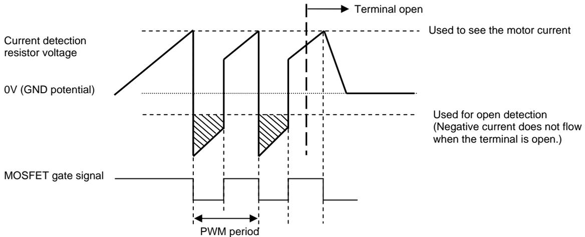
When the current level drops, the difference with the GND potential decreases, making detection difficult. The motor current that can be detected by motor terminal open detection is 0.25A or more with the STK672-612B-E.
