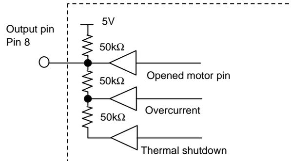
(Configuration of the buffer is open drain.)
