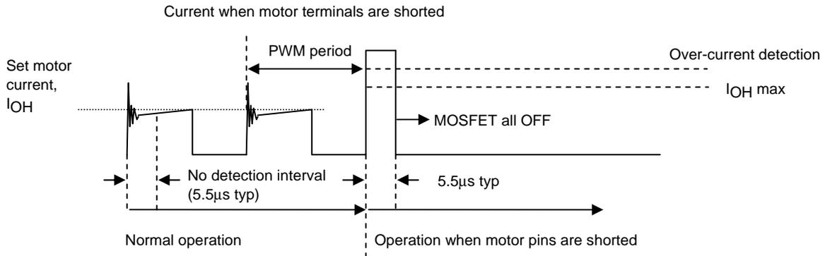
Overcurrent detection begins after an interval of no detection (a dead time of 5.5 $\mu$ s typ) during the initial ringing part during PWM operations. The no detection interval is a period of time where overcurrent is not detected even if the current exceeds  $I_{OH}$ .
