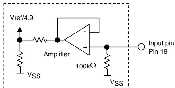
The internal impedance, 100k $\Omega$ , is designed so that the increase in current is prevented while Pin 19 is open.
