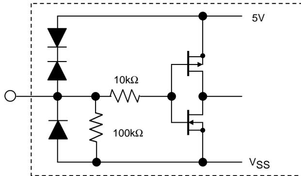
The input pins of this driver all use Schmitt input. Typical specifications at  $T_c=25^\circ\text{C}$  are given below. Hysteresis voltage is 0.3V ( $V_{IHa}-V_{ILa}$ ).
