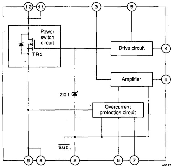
The back surface of the IC is not an insulator, and is effectively at pin 2 potential.
