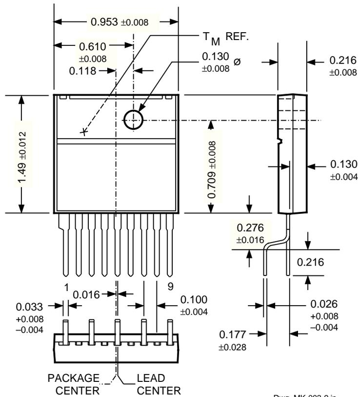
NOTE: Exact body and lead configuration at vendor's option within limits shown.
