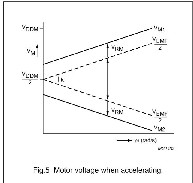
Fig.5 Motor voltage when accelerating.
