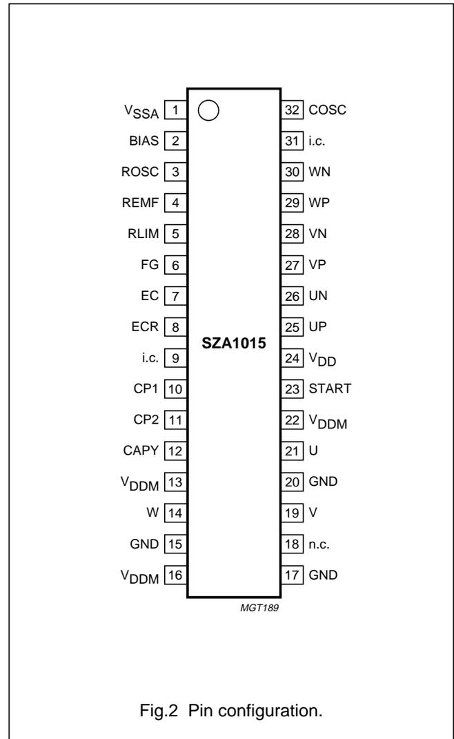
Fig.2 Pin configuration.
