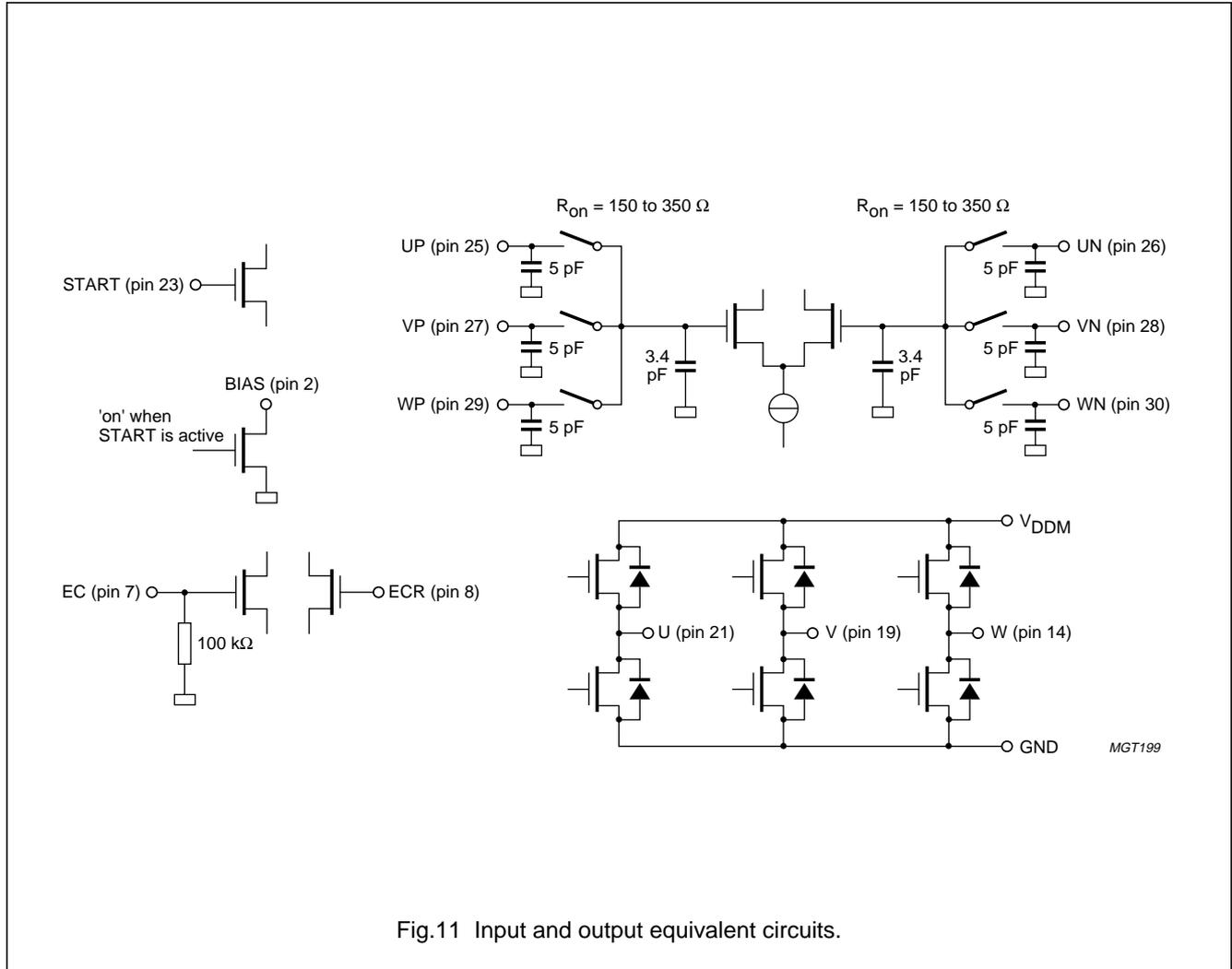
Fig.11 Input and output equivalent circuits.
