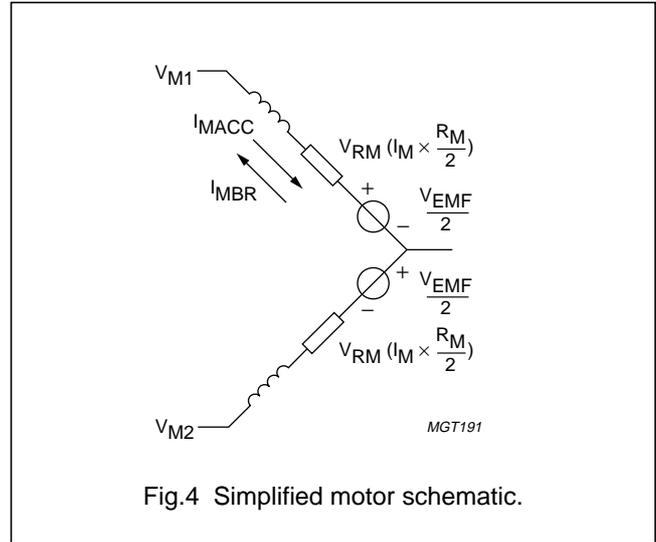
Fig.4 Simplified motor schematic.
