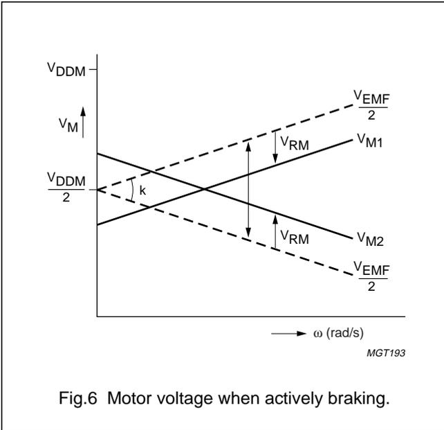
Fig.6 Motor voltage when actively braking.
