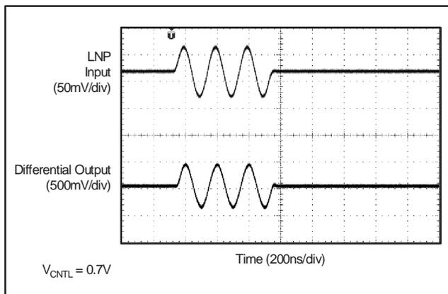
**Figure 67. Before Overload (100mV<sub>PP</sub> Input)**
