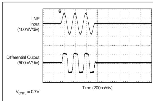
**Figure 69. Overload (240mV<sub>PP</sub> Input)**
