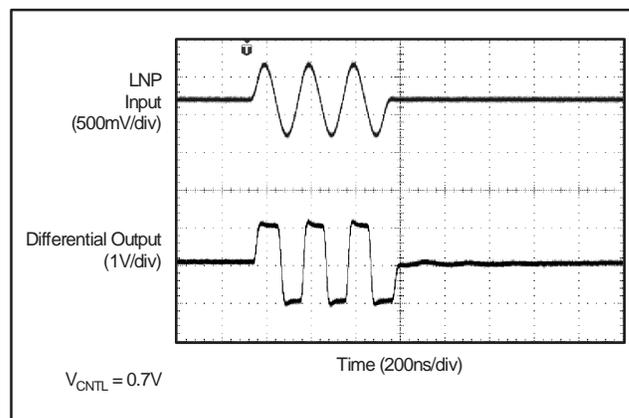
**Figure 70. Extreme Overload (2V<sub>PP</sub> Input)**
