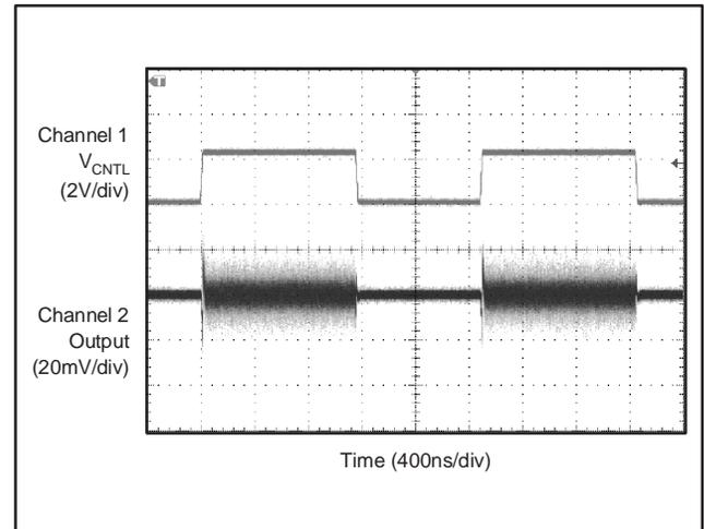
Figure 64. Response to Step Change of  $V_{CTL}$
