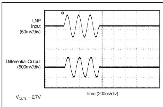
**Figure 68. Approaching Overload (120mV<sub>PP</sub> Input)**
