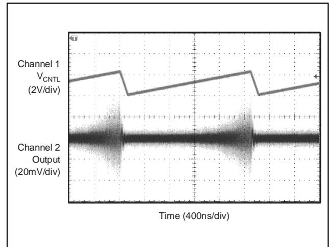
Figure 65. Response to Ramp Change of  $V_{CTL}$
