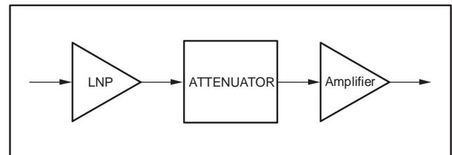
Figure 54. Block Diagram of Older VCA Models
