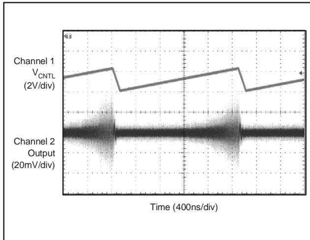
**Figure 38. Response to Ramp Change of  $V_{CNTL}$**
