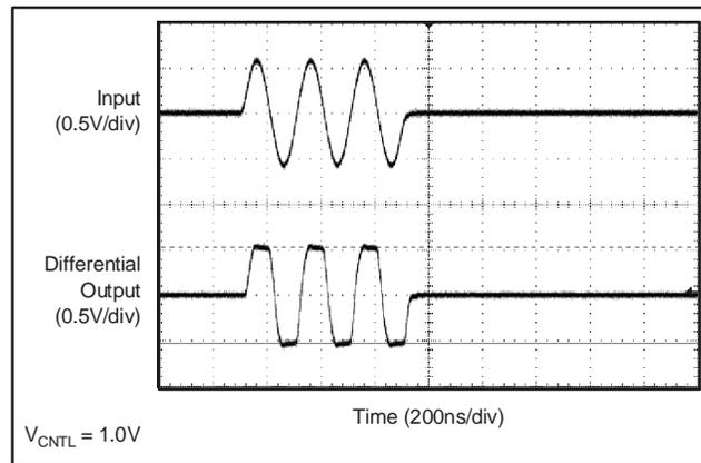
**Figure 42. Overload (1.5V<sub>pp</sub> Input)**
