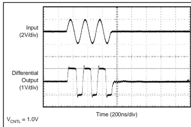
**Figure 43. Extreme Overload (3.8V<sub>pp</sub> Input)**
