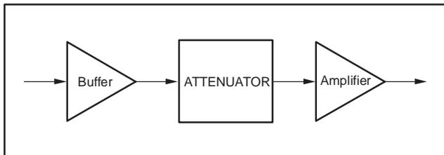
Figure 35. Block Diagram of Older VCA Models
