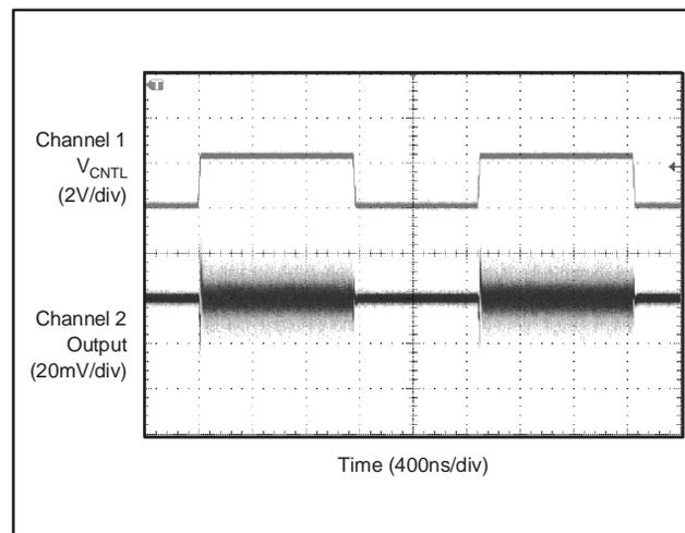
Figure 37. Response to Step Change of  $V_{CNTL}$
