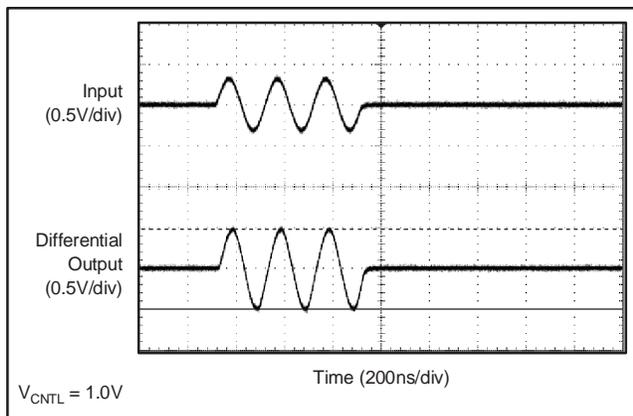
**Figure 40. Before Overload (630mV<sub>pp</sub> Input)**
