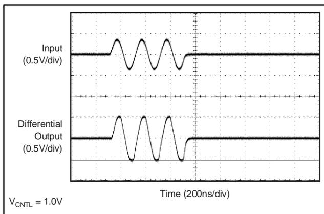
**Figure 41. Approaching Overload (700mV<sub>pp</sub> Input)**
