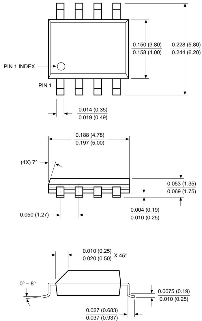
NOTE: ALL DIMENSIONS IN INCHES (IN PARENTHESIS IN MILLIMETERS)
