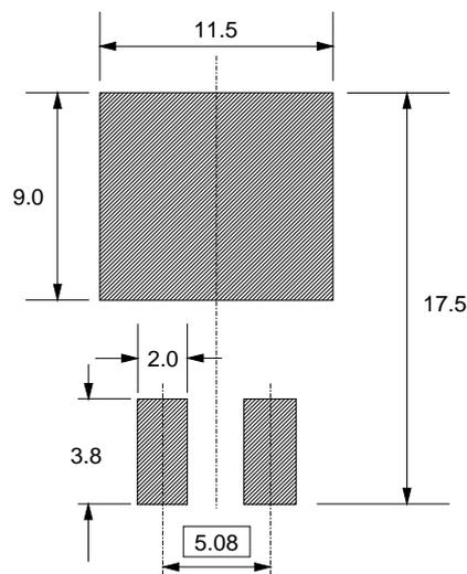
Fig.14. SOT404 : minimum pad sizes for surface mounting.
