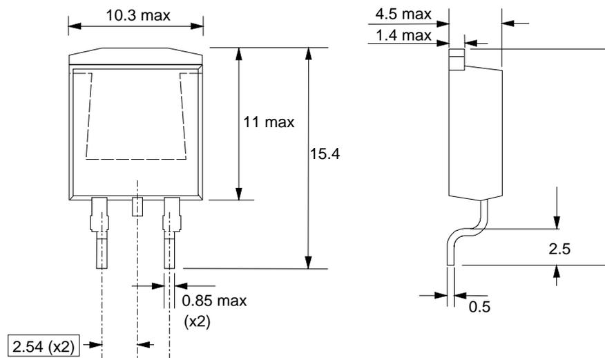
Fig.13. SOT404 : centre pin connected to mounting base.
