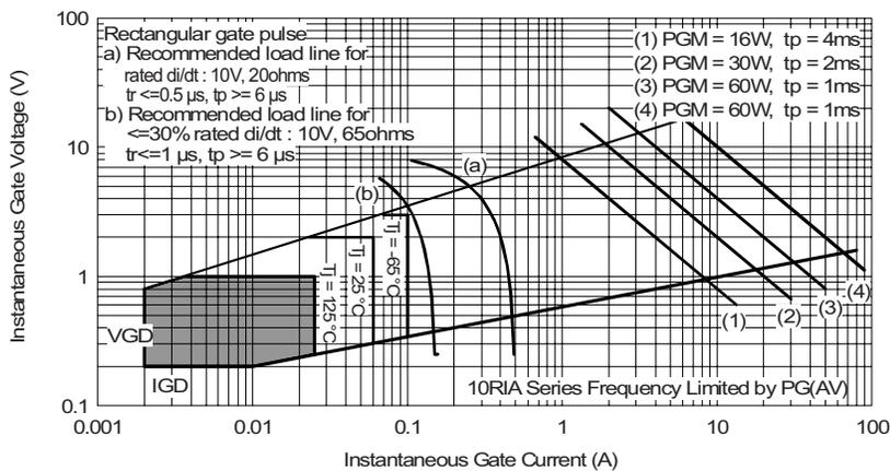
Fig. 9 - Gate Characteristics
