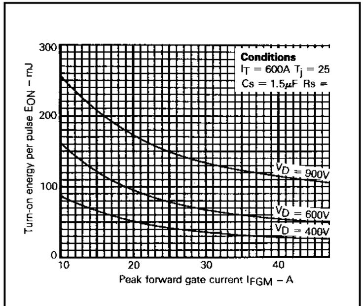
Fig.10 Turn-on energy vs peak forward gate current
