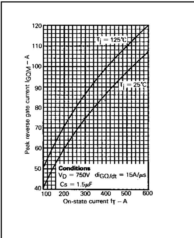
Fig.25 Peak reverse gate current vs on-state current
