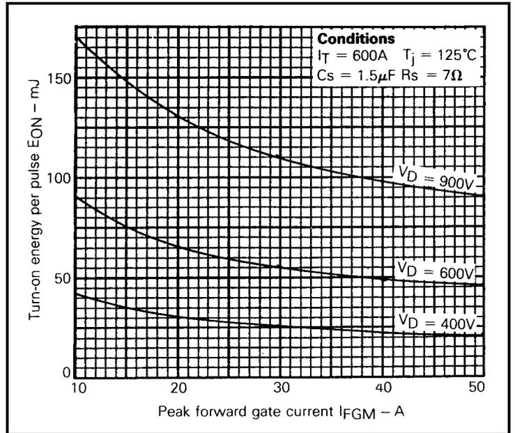
Fig.12 Turn-on energy vs peak forward gate current
