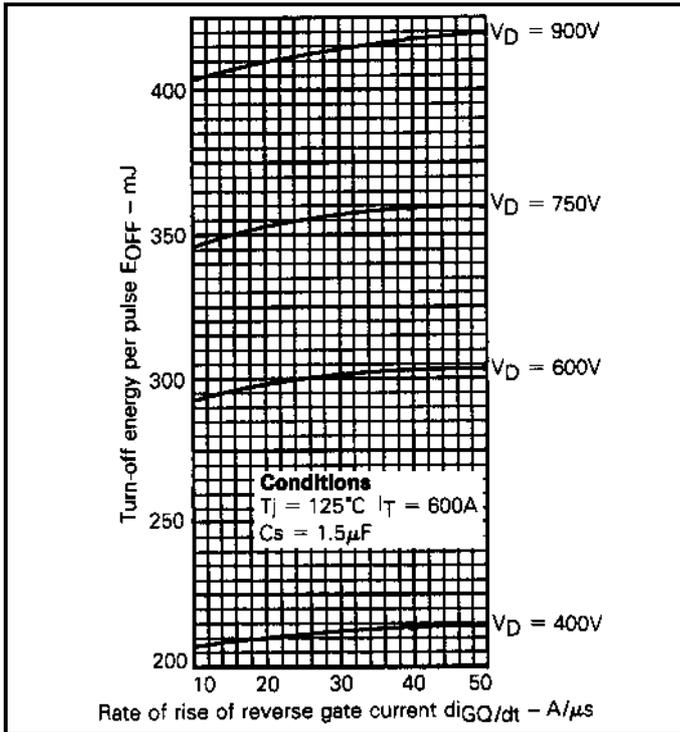
Fig.19 Turn-off energy vs rate of rise of reverse gate current
