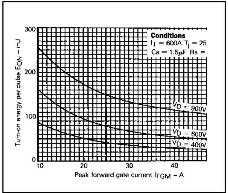
Fig.9 Turn-on energy vs peak forward gate current
