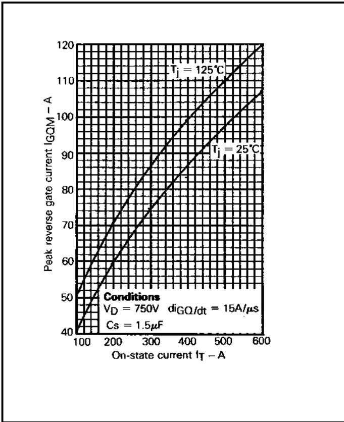
Fig.24 Peak reverse gate current vs on-state current
