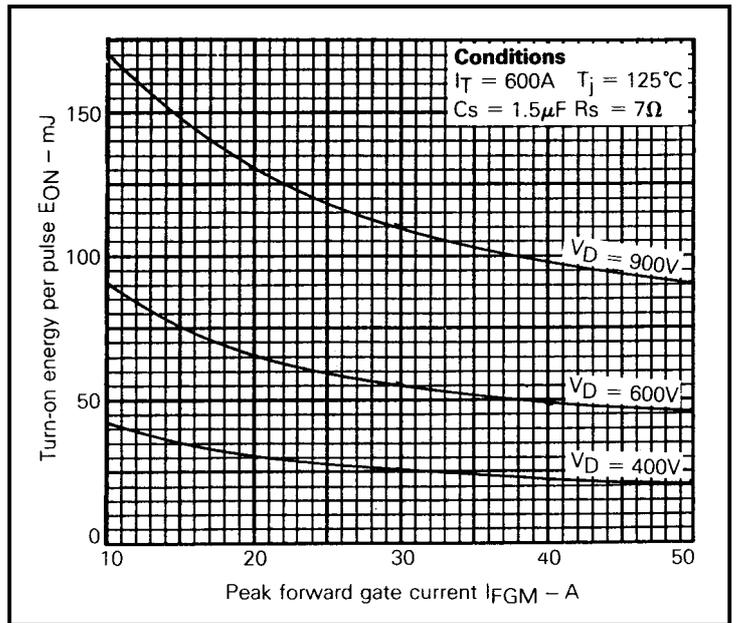
Fig.11 Turn-on energy vs peak forward gate current
