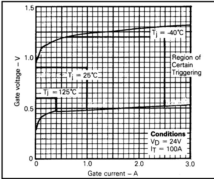
Fig.1 Gate characteristics
