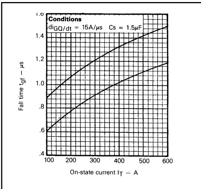
Fig.22 Fall time vs on-state current
