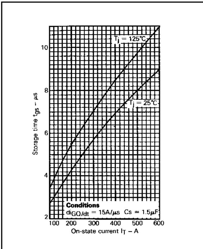
Fig.20 Storage time vs on-state current
