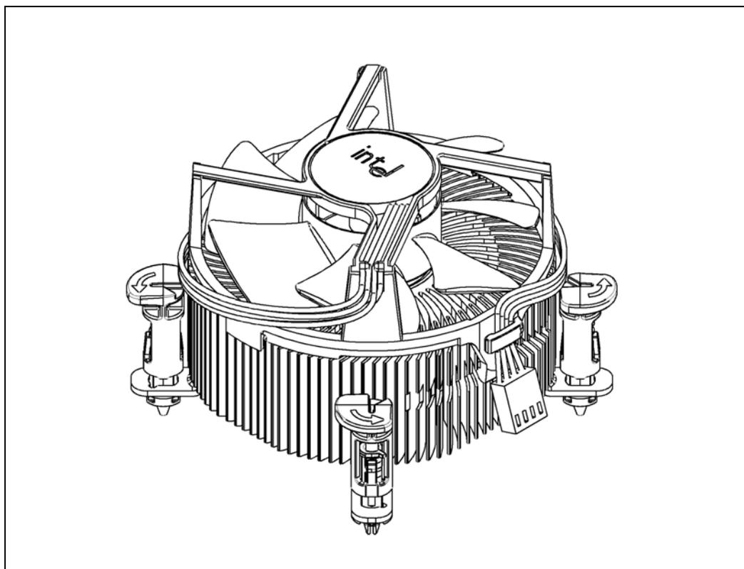
**NOTE:** The airflow of the fan heatsink is into the center and out of the sides of the fan heatsink.
