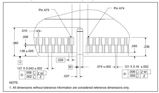
Figure 37. S.E.C.C.2 Packaged Processor Substrate — Keep In Zones
