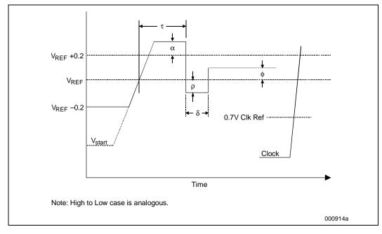
Figure 15. Low to High AGTL+ Receiver Ringback Tolerance
