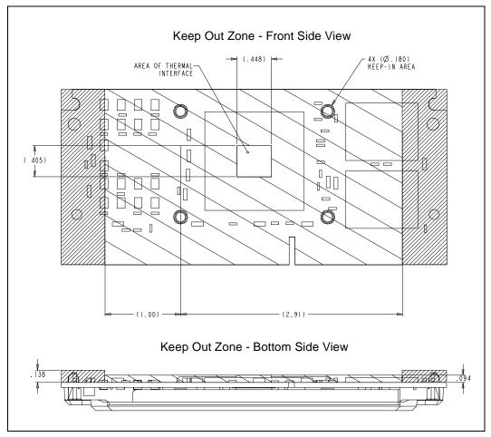
Figure 38. S.E.C.C.2 Packaged Processor Substrate — Keep-Out Zone
