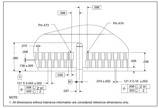
Figure 27. S.E.C.C. Packaged Processor Substrate — Edge Finger Contact Dimensions, Detail A
