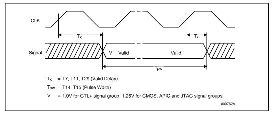
Figure 8. System Bus Setup and Hold Timings
