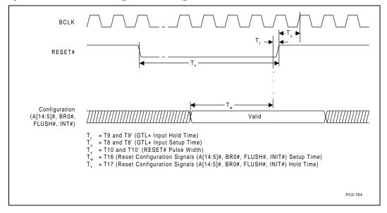
Figure 10. Power-On Reset and Configuration Timings
