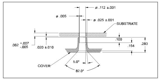
Figure 33. S.E.C.C.2 Packaged Processor Assembly — Side View
