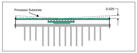
Figure 41. Substrate Deflection Toward the Heatsink
