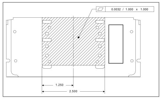
Figure 26. S.E.C.C. Packaged Processor Substrate — Edge Finger Contact Dimensions
