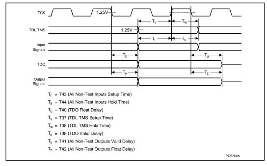
Figure 12. Test Reset Timings
