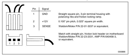
Table 38. Fan Heatsink Power and Signal Specifications
