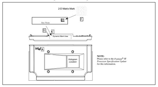
Table 31. Description Table for Processor Markings (S.E.C.C.2 Packaged Processor)
