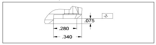
Figure 35. S.E.C.C.2 Packaged Processor Substrate — Edge Finger Contact Dimensions
