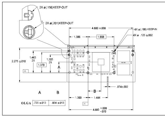
Figure 30. S.E.C.C.2 Packaged Processor Assembly — Primary View
