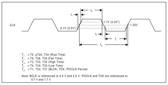
Figure 7. System Bus Valid Delay Timings
