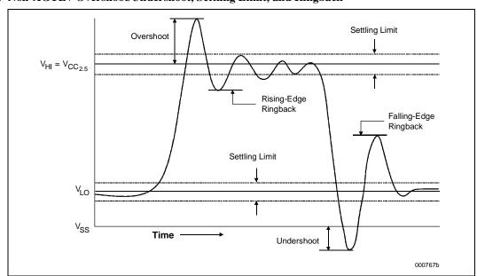
Figure 16. Non-AGTL+ Overshoot/Undershoot, Settling Limit, and Ringback
