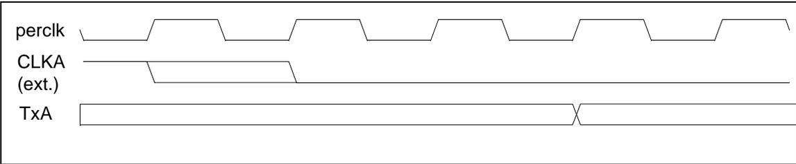
Figure 12-6. Synchronous Serial Data Transmit Timing with External Clock
