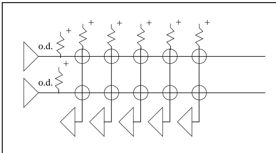
**Figure 4-2. Using Open-Drain Outputs for Key Scan**
