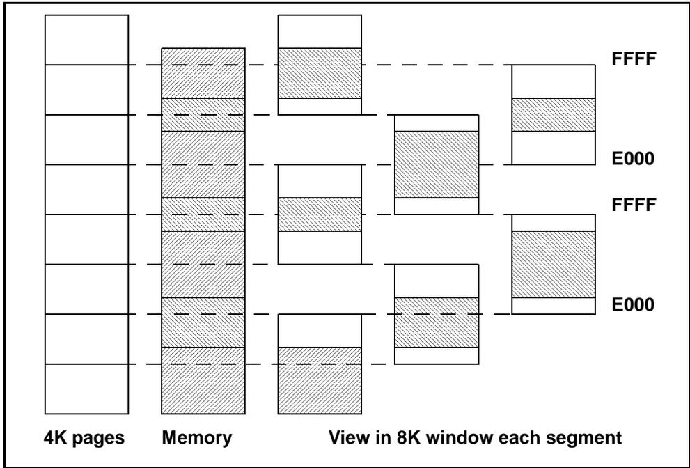
*Figure 8-4. Compilation of Code Segments in Extended Memory*
