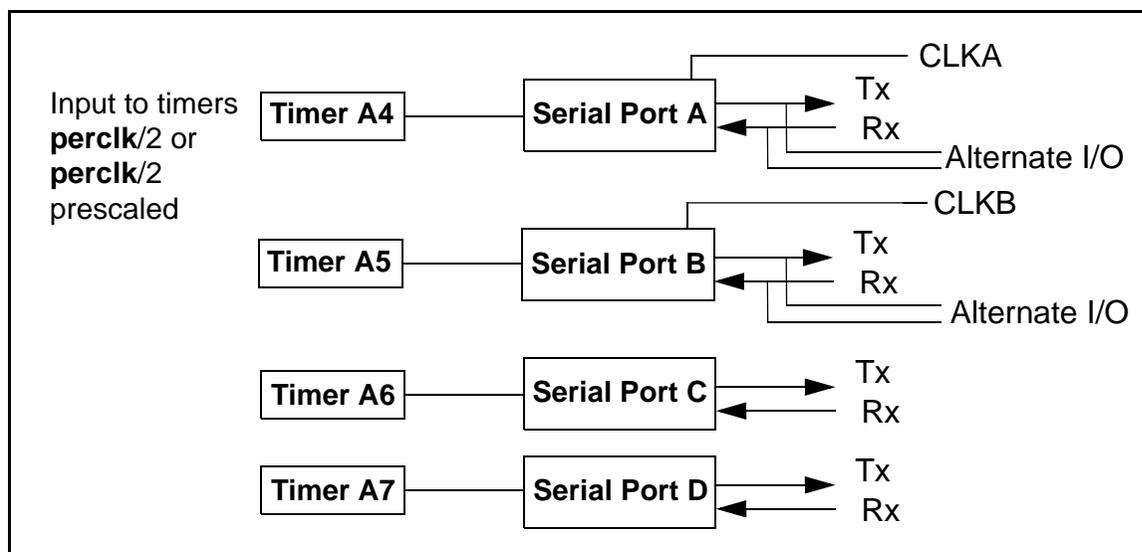
**Figure 12-1. Block Diagram of Rabbit Serial Ports**
