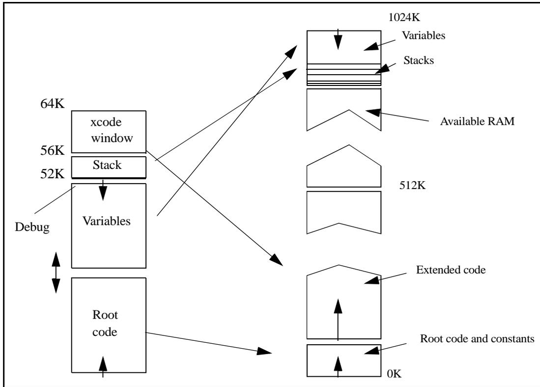
**Figure 8-3. Example of Memory Mapping and Memory Usage**
