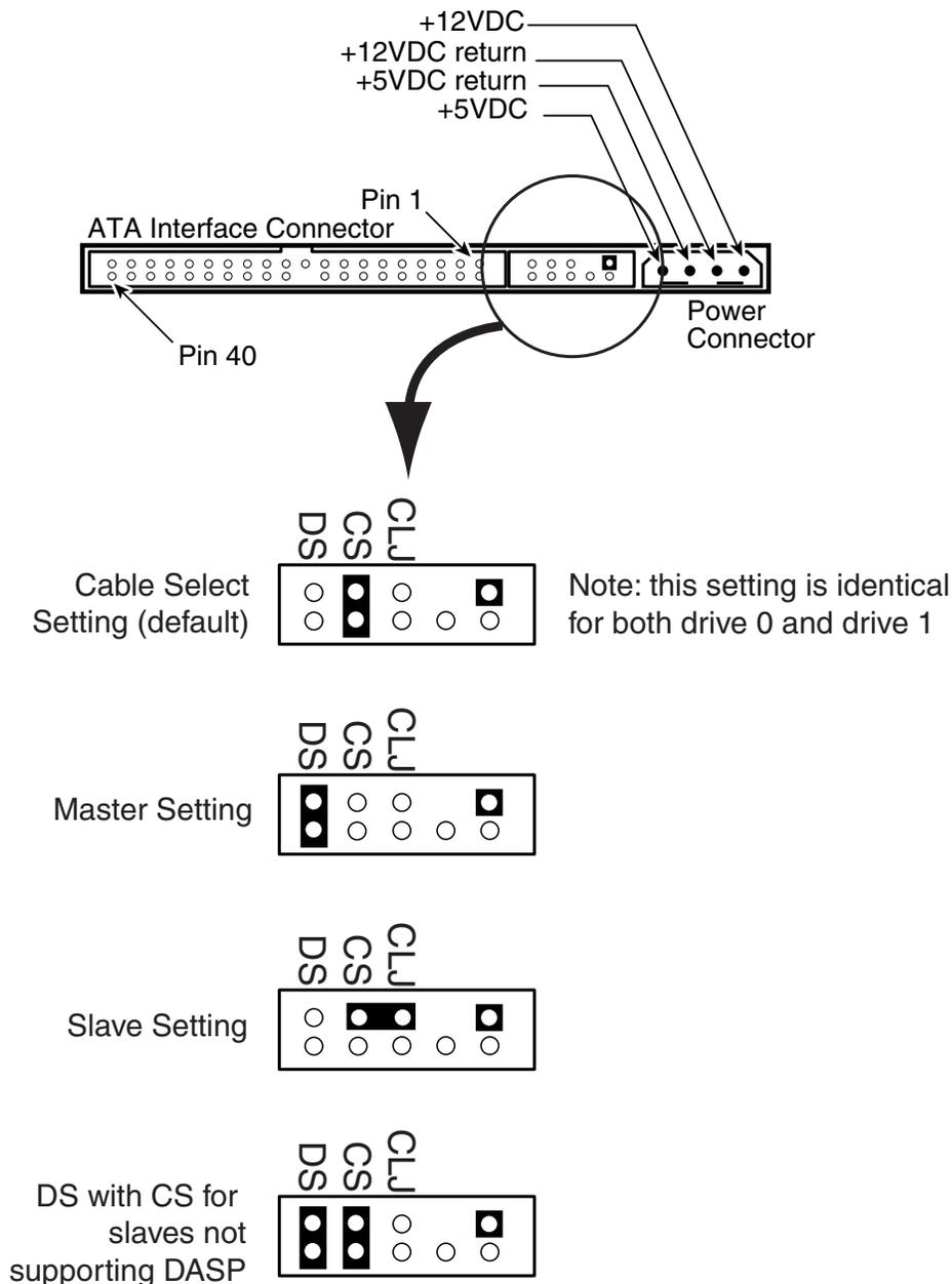
Figure 3-4 Jumper Locations on the ATA Interface Connector
