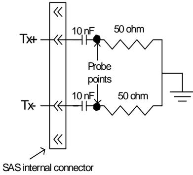
**Figure 22. Zero-length test load**
