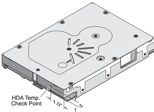
Figure 10. Location of the HDA temperature check point
