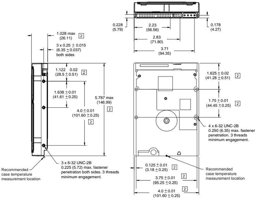
Figure 5. Mounting dimensions—top, side and end view
