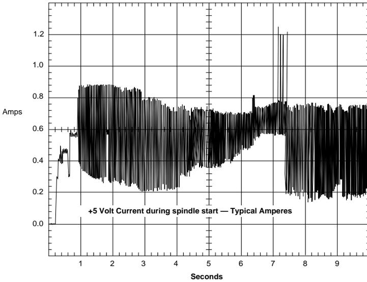
Figure 1. Typical 5V startup and operation current profile
