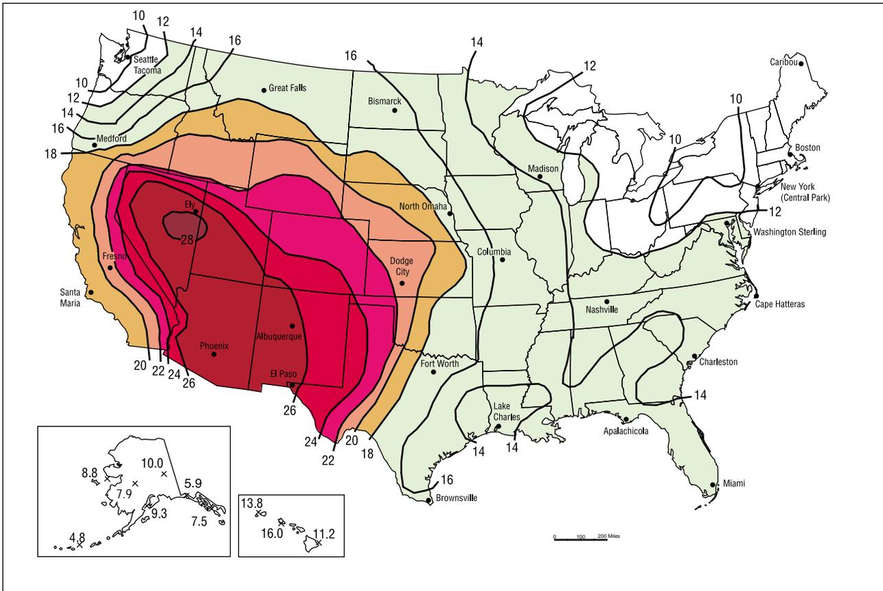
Values for average direct solar radiation for locations in the USA are shown in Figure 7. For conversion purposes, to determine a derating factor from Figure 6 from the information by location from Figure 7, 1 MJ/m<sup>2</sup> over a 24-hour period is equivalent to 11.6 W/m<sup>2</sup>.
