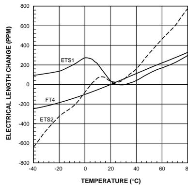
Figure 5 – Electrical Length Change vs. Temperature
