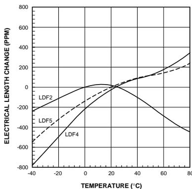
Figure 4 – Electrical Length Change vs. Temperature
