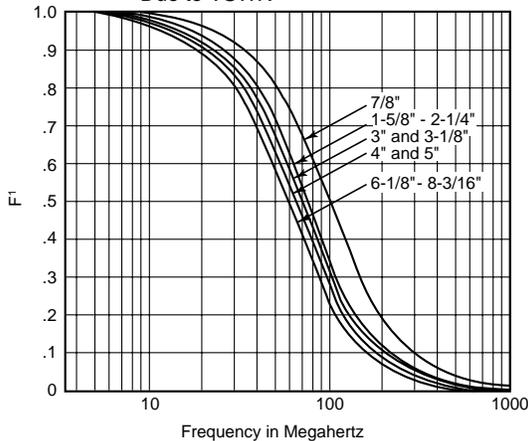
Andrew average power ratings are based on a VSWR of 1.0, atmosphere pressure and ambient temperature of 40°C (104°F).
