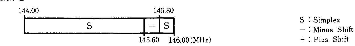
The ARS function is disabled at the factory. It is toggled on and off by pressing F/M, RPT, F/M and RPT (that is, each key, twice alternately). Pressing F/M and RPT the first time displays the repeater
